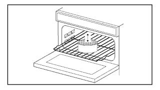
When cooking cakes, pastry, scones, bread etc., place the tins or baking trays centrally on the shelf directly below the element.  DO NOT place dishes or baking trays directly onto the oven base as it becomes very hot and damage may occur.
